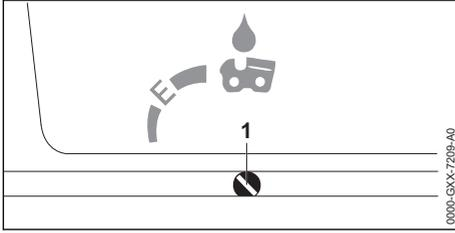
The oil feed rate is suitable for most applications when the oil pump adjusting screw (1) is in position E (Ematic).
